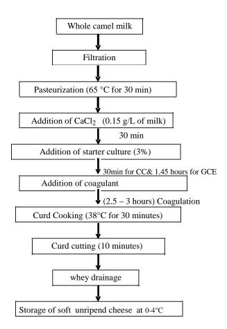
**Figure 1.** Flow diagram for the manufacture of soft unripened cheese from camel milk.
