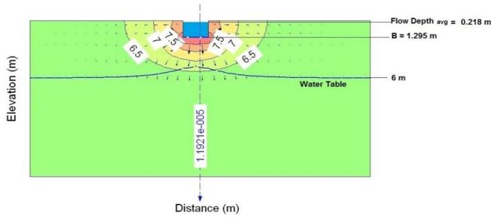
**Figure. 2.4:** Flownet of 1 R Qaiser Minor for Reach IV (Seepage =  $1.192 \times 10^{-5}$  m<sup>3</sup>/sec/m)
