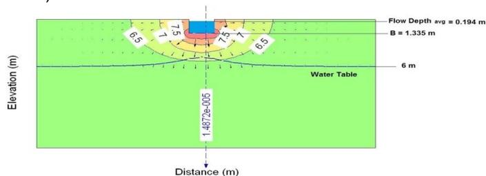
**Figure. 2.1:** Flownet of 1 R Qaiser Minor for Reach I (Seepage =  $1.487 \times 10^{-5} m^3/sec/m$ )
