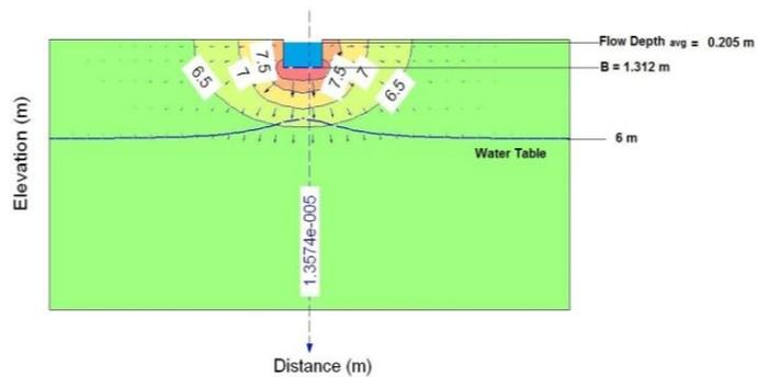
**Figure.2.2:** Flownet of 1 R Qaiser Minor for Reach II (Seepage =  $1.357 \times 10^{-5} m^3/sec/m$ )
