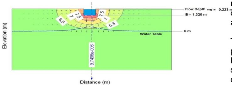
**Figure. 2.5:** Flownet of 1 R Qaiser Minor for Reach V (Seepage =  $9.749 \times 10^{-6}$  m<sup>3</sup>/sec/m)
