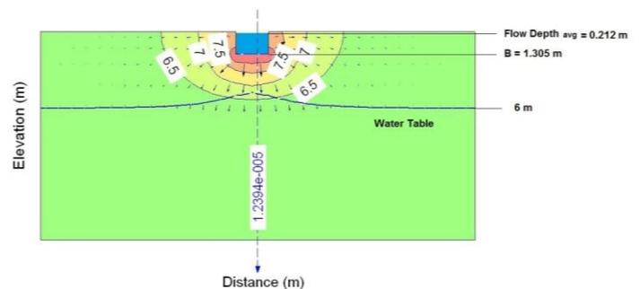
**Figure.2.3:** Flownet of 1 R Qaiser Minor for Reach III (Seepage =  $1.239 \times 10^{-5} m^3/sec/m$ )
