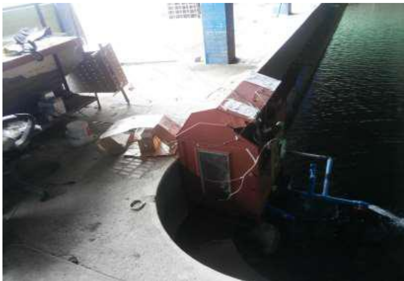
Figure 1. Hot spring incubator operating on automatic turning.
