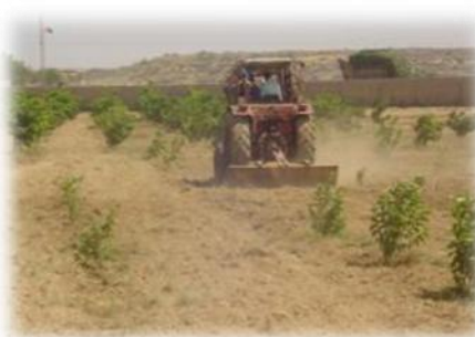
Figure 1b: Rough Levelling with Rear Blade
