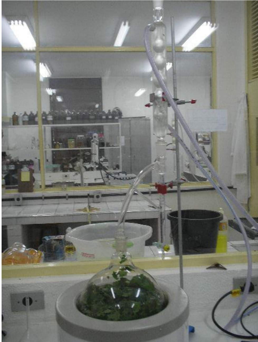
Figure 5. Essential oil extractor, model Clevenger do LPPN— URCA - Crato-CE.
